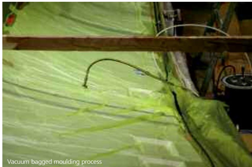
Vacuum bagged moulding process
