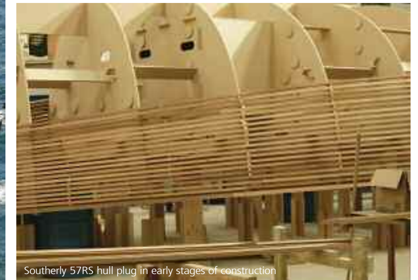
Southernly 57RS hull plug in early stages of construction
